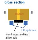
The AVZ comprises a central belt that runs continuously. A lift-up frame is mounted beside this belt frame which extends along the entire zone length on both sides. When the lift up is in a low position, the items are conveyed on the belt. If raised, it is held in the zone.
