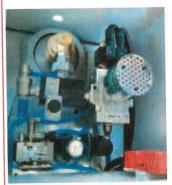
The double body device, guarantees the clutch stop in full safety, under any emergency condition.
