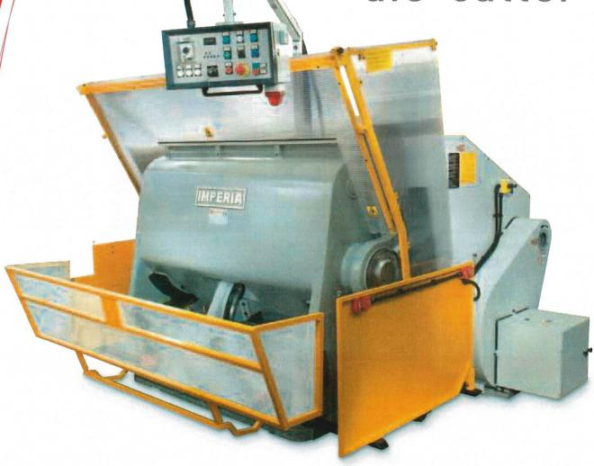
MPERIA platen die-cutters, universally known for their strong power, are suitable for die-cutting, creasing and embossing works on flat, corrugated or laminated cardboard sheets.
