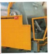
These are placed to prevent any access into the machine parts and to guarantee the total operator protection, allowing the stop of the movable plane motion, at any time.
