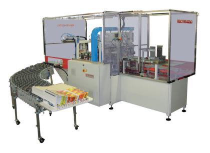
Automatic machine to thread and glue one flat elastic band onto laying flat agenda and diary cases.
