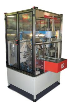
Half-automatic machine to apply one flat elastic band onto spiral note books by Nr. 02 eyelets or rivets.
