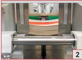
It is 50 mm (2") height and ensures a gentle and straight falling of the books in the main stacking station. Its grids are pneumatically moved, thought one cylinder mechanically connected to both.
