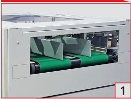
Conveys the products inside the machine, the group of side guides build on it allign the products before launching.
