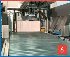
PRESSING - STRAPPING: The bundle that has been driven to the exit, will find at its ends the boards that has been driven to the exit, will find at its ends the boards that has been previously manually positioned from the operator. Through the "two hands" control the pressing and the strapping are activated (pressure weight and strap tension can be adjusted). The bundle is then ready to be picked up.
