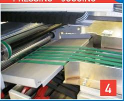
PRESSING - JOGGING: The Rotodò, has a built in pressing station composed by two steps, where the first two rollers with diameter of 80 mm takes the air out and the following two with diameter of 160 mm deliver a high pressure to the paper. The elimination of the air between the pages ensure an easier handling in the following processing. After the second pressing, the signatures are shingled and jogged by means of the harmonious movement of the eccentric jogger.
