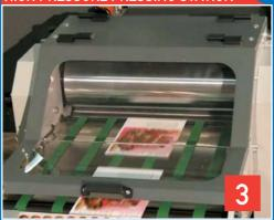
HIGH PRESSURE PRESSING STATION (OPTIONAL): The additional pressing station. placed between the infeed conveyor and the stacker, allows a perfect pressing even with the more difficult papers. The a.m. is made out of two pressing rollers with a diameter of 190 mm easily adjustable by mean of hand-wheels.
