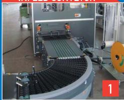
INFEED CONVEYOR: Adjustable in height to be connected to any type of folder or at the exit of printing machines with signatures delivery. The round belt conveyor is endowed with a side adjustment to allow the positioning of the single signature or continuous stream in the center of the machine.
