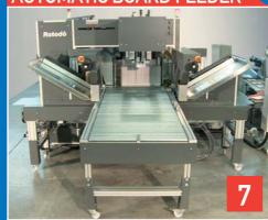
AUTOMATIC BOARD FEEDER (OPTIONAL): This application allows to optimize the Rotodò automation, helping the operator and increasing the productivity possibilities.
