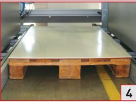
Once the complete layer have been off-loaded, the slip-sheet is automatically stored into a high capacity magazine which is easily accessible to the operator. The magazine is endowed with side joggers to ensure a perfect stacking of the slip-sheets. This guarantees the possibility to reuse the slip-sheets.
