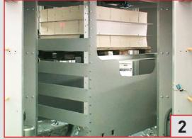
The pallet is lifted until the off-loading position is reached enabling the moveable roller's conveyor to come close to the top layer of the pallet and to clamp the slip-sheet transferring it with the products on its gravity conveyors. The complete pallet is then rotated of 180° to reach the proper product orientation before repeating the off-loading process with the next layer.
