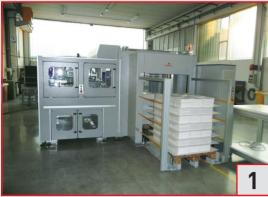
The pallet of products is positioned on a motorized conveyor where the height of the pallet is checked. The conveyor is made of chain planes that guarantee stability while the pallet is transported inside the **VENUS**.
