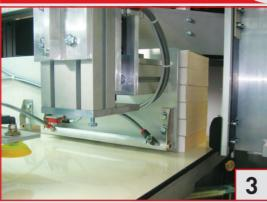
The layer of products that has been moved on the gravity roller plane is then divided in rows by pushing them one by one on the delivery conveyor. In order to prevent damages or markings to the products, the row pushing station is endowed with a blowing system to create an "air cushion" underneath the product.
