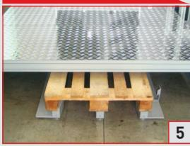
The empty pallet is put down from the elevator on the motorized chain conveyor and conveyed in the pallet delivery area to be easily removed by hand or by means of a pallet lifter.
